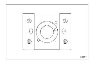
(2) Assembly tool for O-ring and kin-ring.
